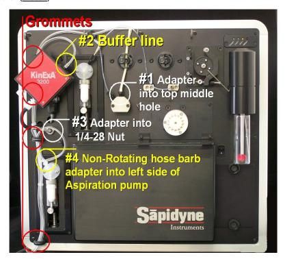
Figure 1: Buffer Waste Connection routing diagram.
