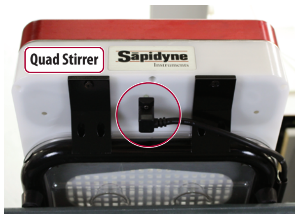
Figure 4. Serial cable connection to the Quad Stirrer.
