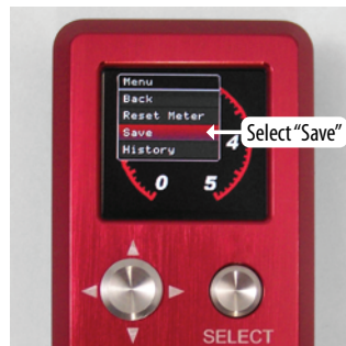
Figure 7. Save the information to keep a record of lamp replacements and power levels.
