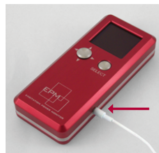
Figure 3. Plug the sensor into the EPM.
